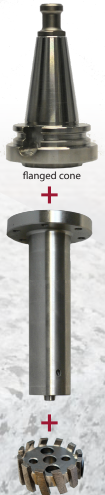
3. CROWN MILL Ø30 Cut from 60 to 200 mm RPM: 4200 - 4800 Feed: 250 - 500 mm/min Each Step: 1 - 3 mm
